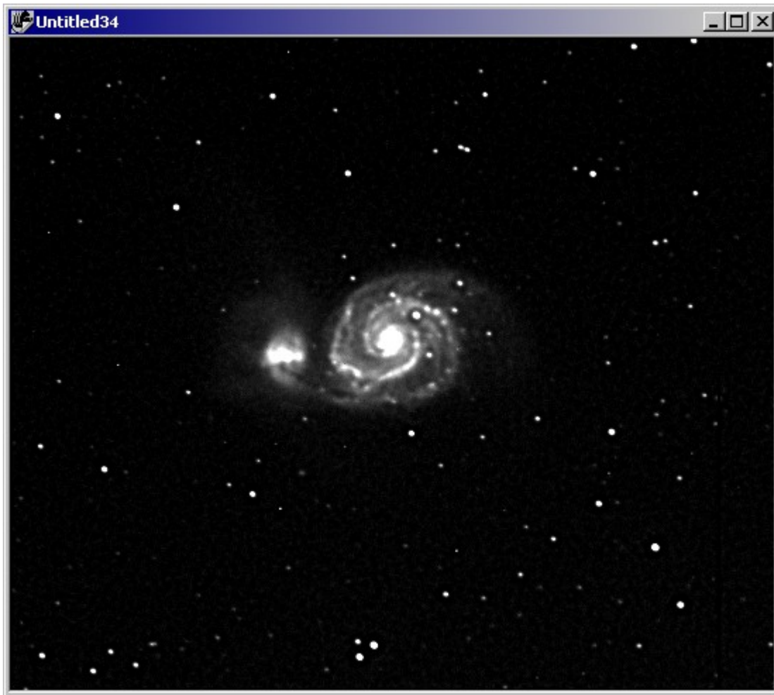
Figure 44: An example of too many iterations, or an overly large sigma value.
