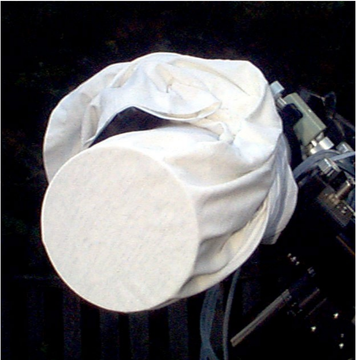
Figure 19: Using a T-shirt to take a flat in daylight. Be sure to point the scope away from bright sources of light.
