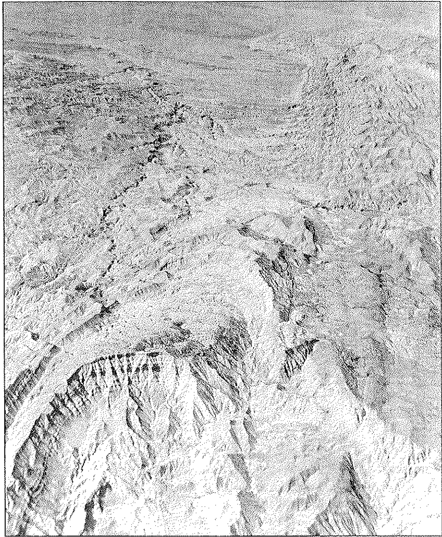
FIGURE 2-7 Denuded pitching anticline in typical structures of the Folded Zagros Mountains of western Iran. In such subsurface folds are found the great petroleum reservoirs of the area. Compare with Figure 8-6, which shows salt domes that also form oil-reservoir structures.
